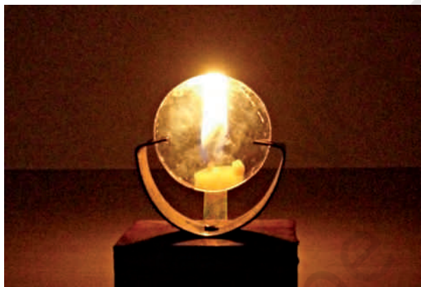
Fig. 11.26 Virtual image formed by the convex lens
