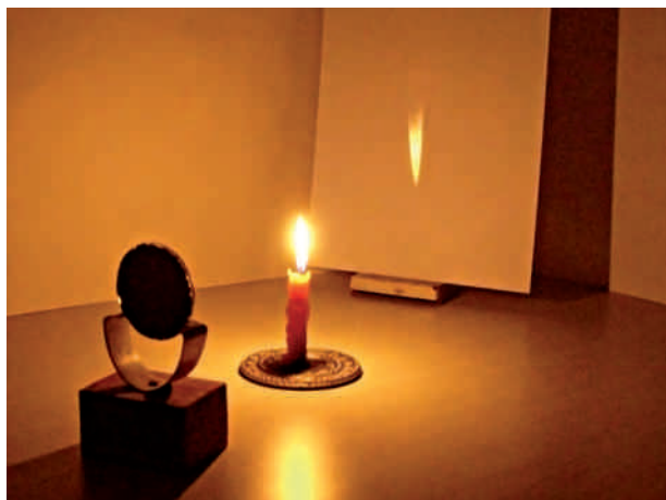
Fig. 11.15 Real images formed by a concave mirror
