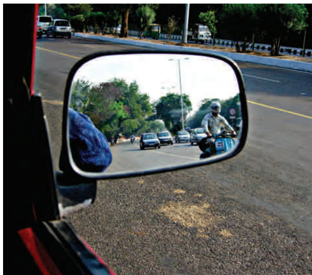
Fig. 11.20 Convex mirror as side view mirror
