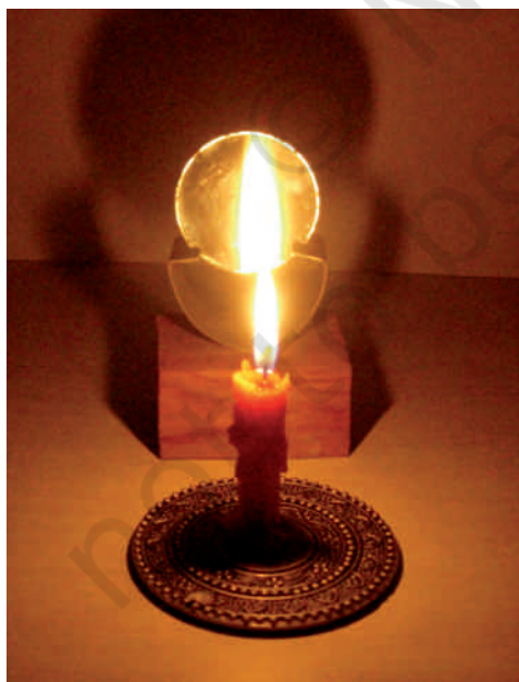
Fig. 11.16 Virtual image formed by a concave mirror
