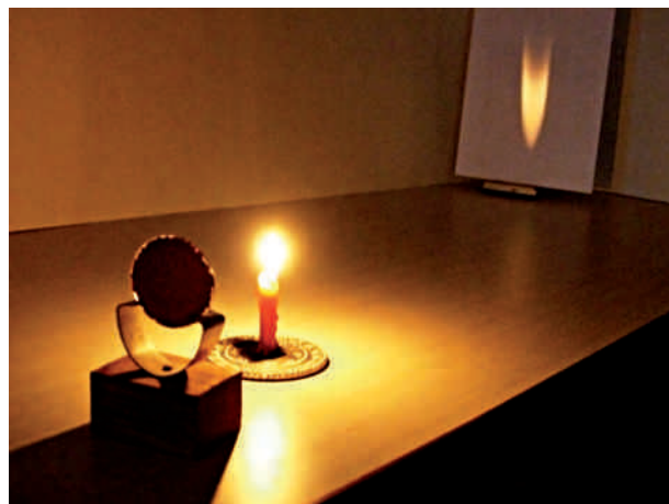
Fig. 11.15 Real images formed by a concave mirror
